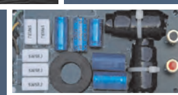
18dB EPOXY BOARD, HIGH CURRENT, HIGH TEMPERATURE CROSSOVER WITH POLYSWITCH PROTECTION
