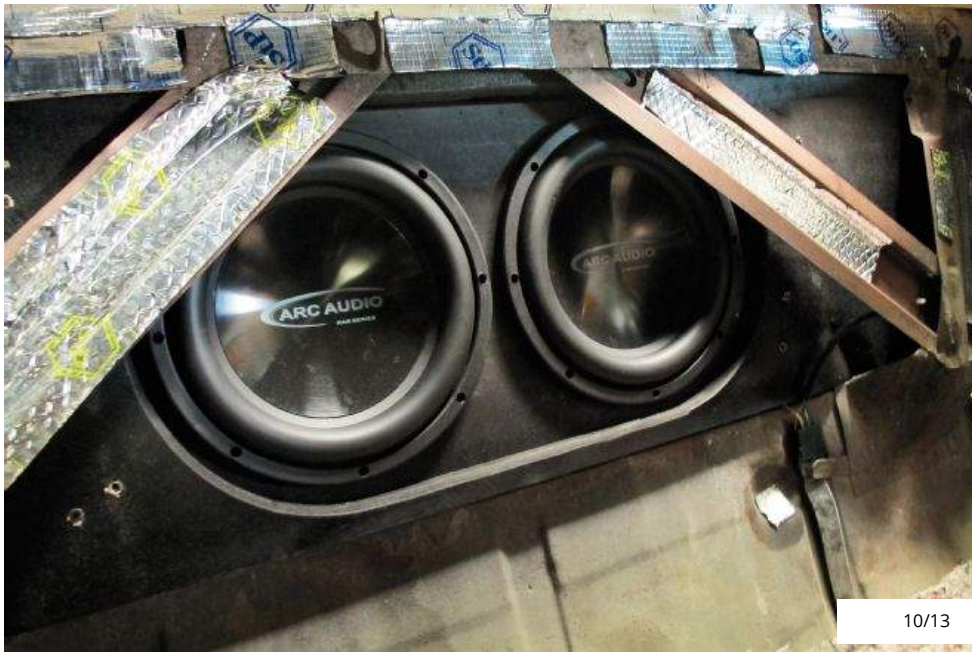
09 ...two 10-inch Arc Audio XDi subwoofers enclosed behind the rear seat back...
