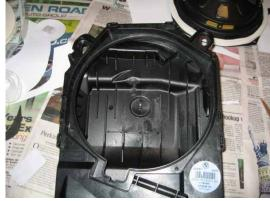
This is the box with the factory sub removed, ready for the SWS shallow woofer.
