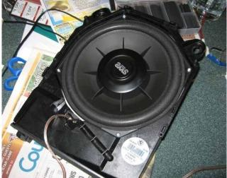
The standard box under the BMW seat fits Earthquake's SWS 8 inch shallow woofer easily and with hardly any modification.
